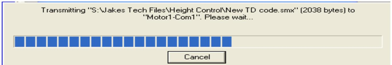
Once the program is finished close out of the SMI software. Power cycle the Height Control Box. The AVHC motor should have a green led light lit indicating a ready state. In order to check the Height Control motor for proper functionality jump the Start Input Connector on the back of the AVHC box. This will trigger the on command to tell the Lifter Station to come down, and sense the material.
